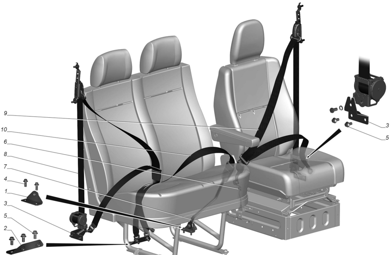
Fig 1 Installation seat belts
