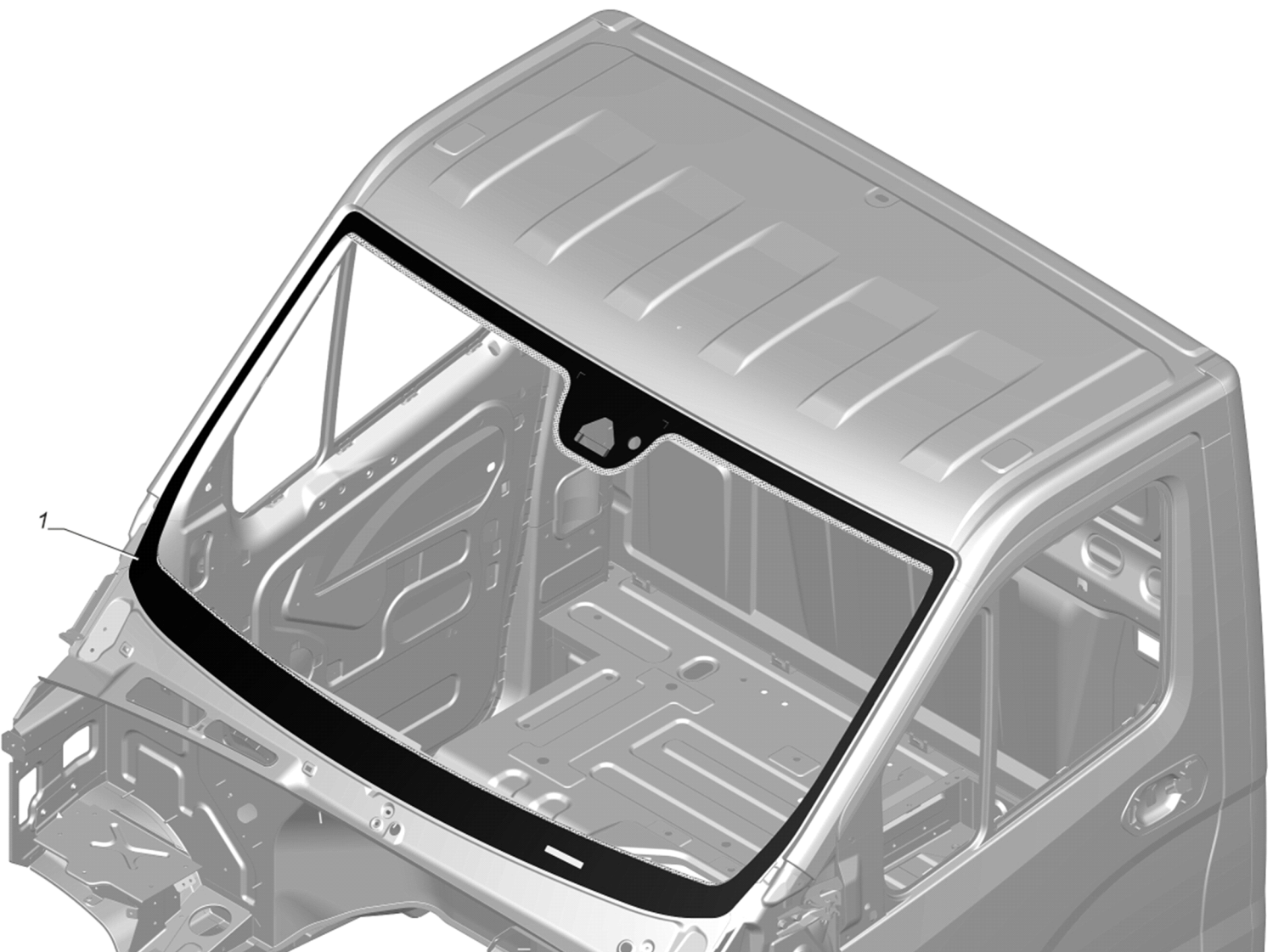
Fig 1 Installation the windshield glass
