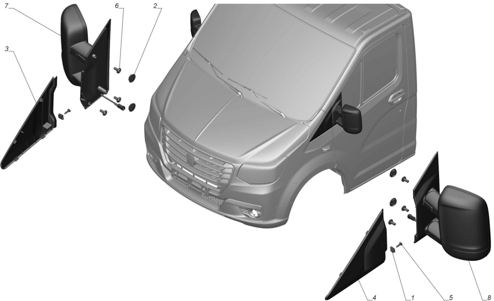
Fig 1 Installation of rear-view mirrors
