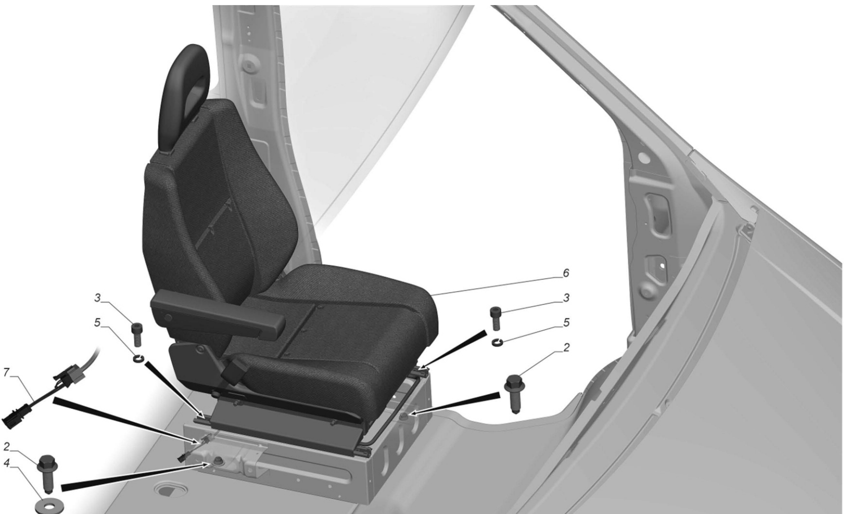
Fig 1 Installation the Driver's Seat
