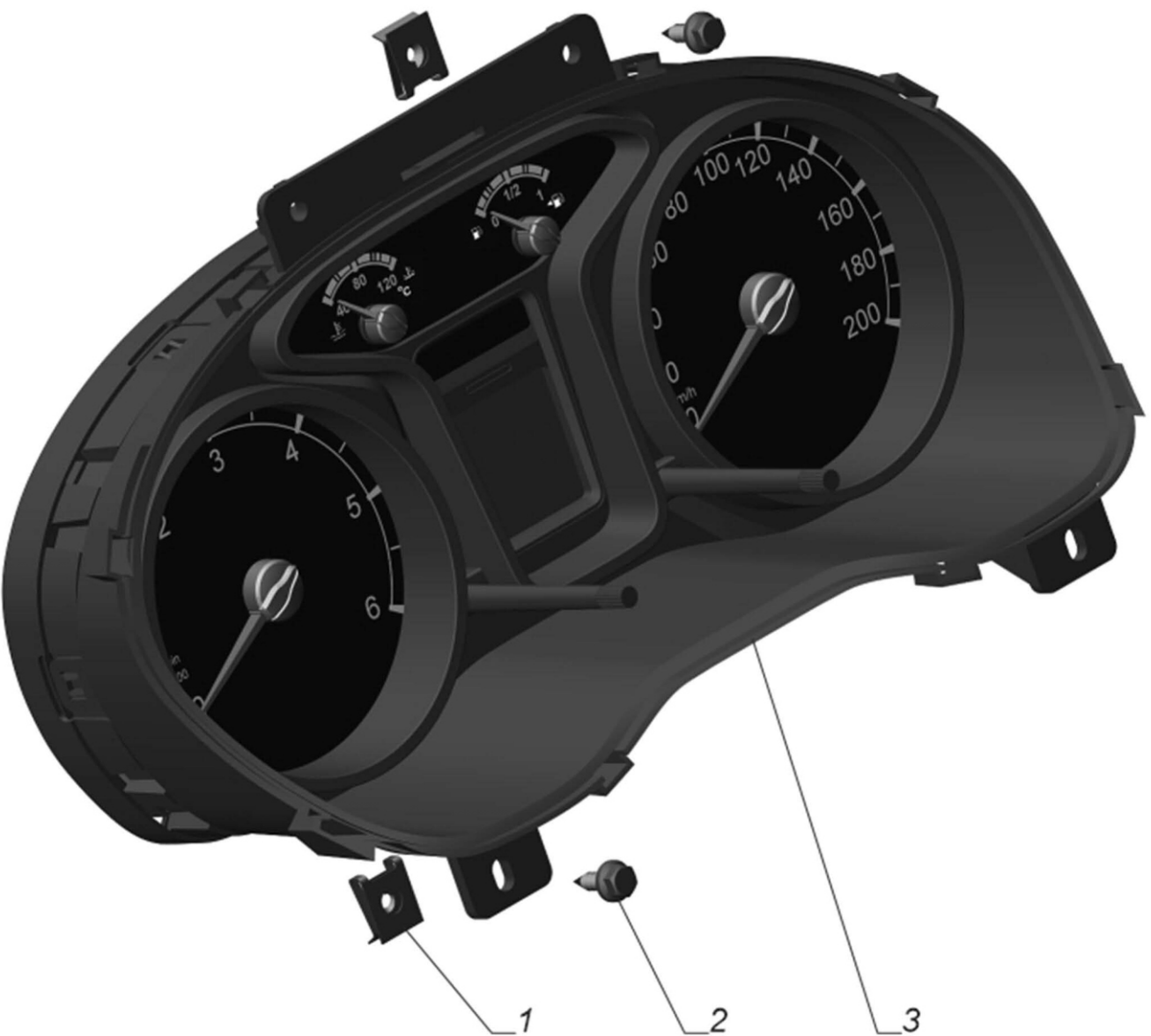
Fig 1 Installation the instrument cluster
