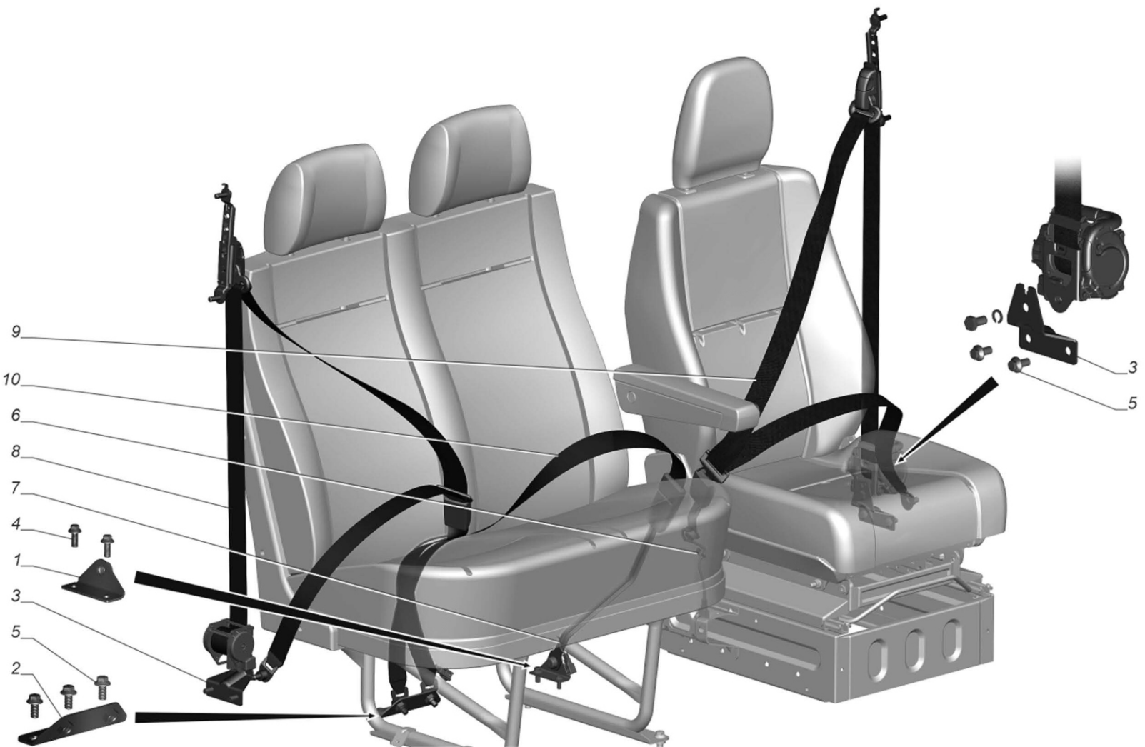
Fig 1 Installation seat belts
