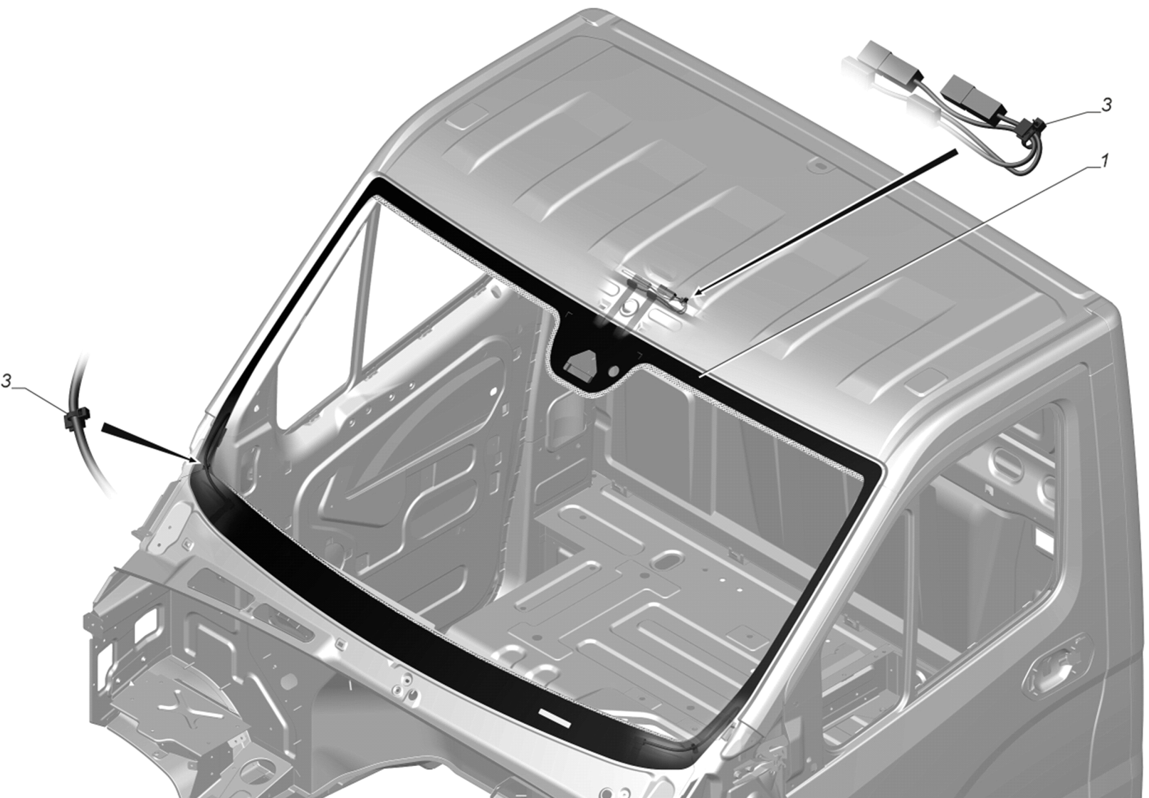
Fig 1 Installation the windshield glass
