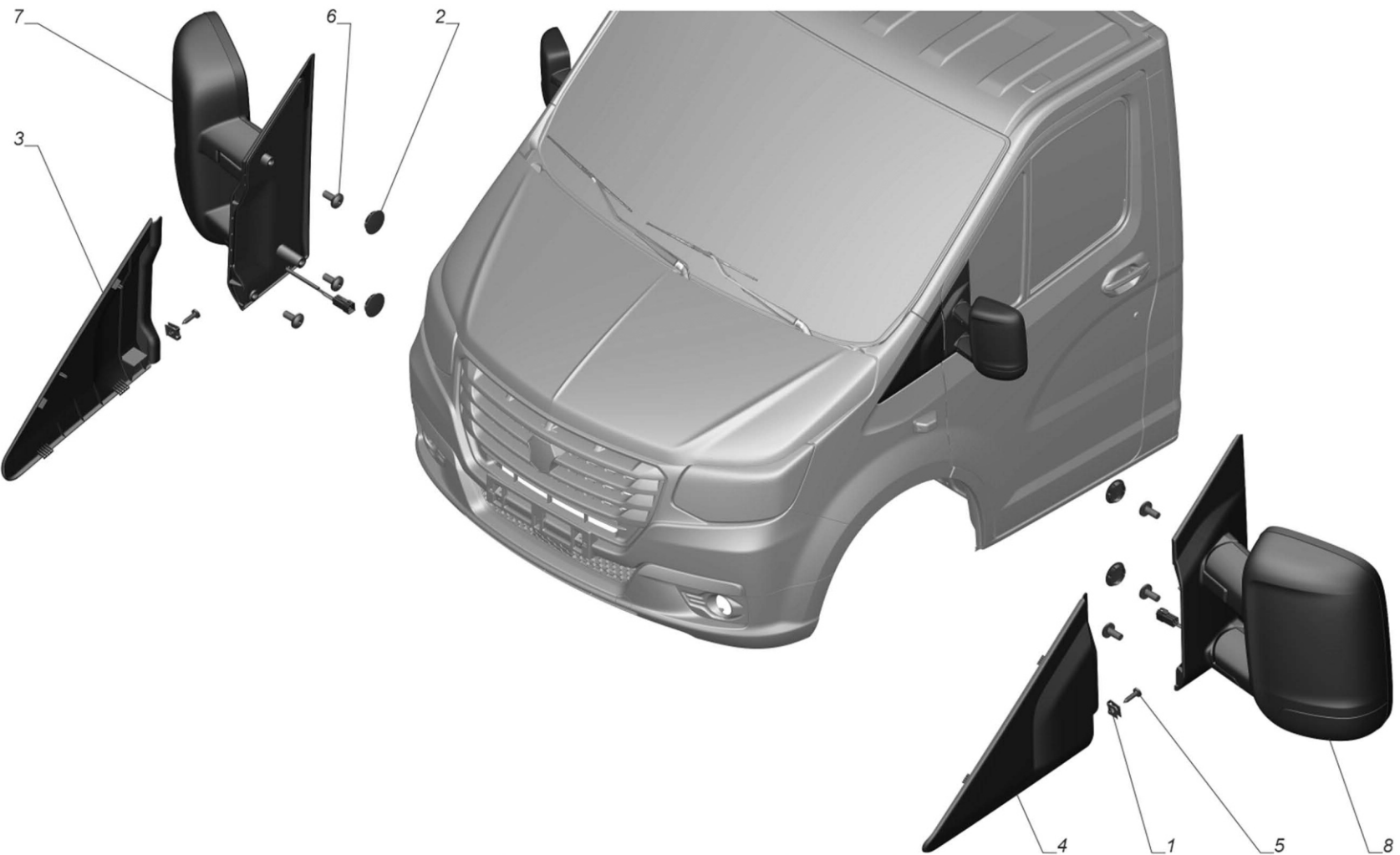
Fig 1 Installation of rear-view mirrors
