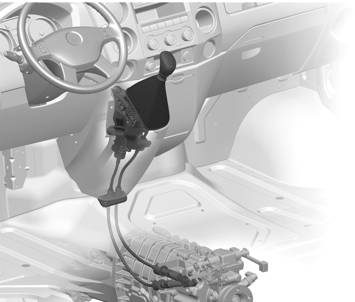
Fig 1 Installation of the master support with cables
