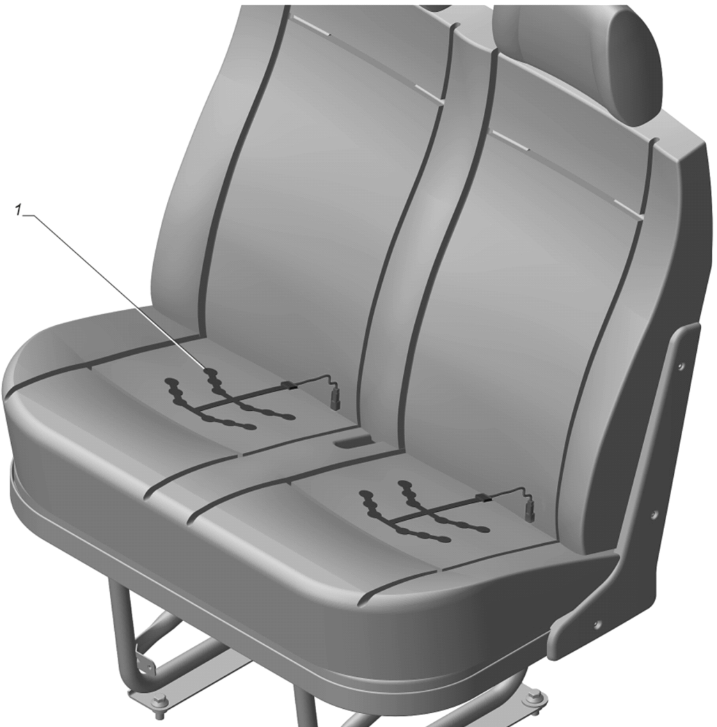
Fig 1 Installation seat occupancy sensors
